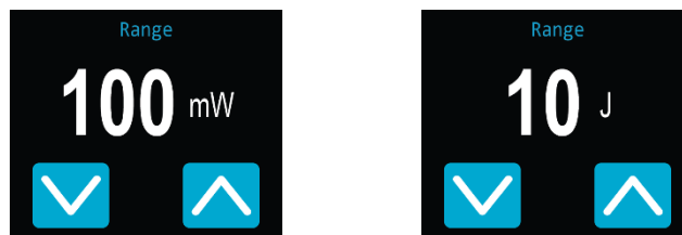
Figure 7. Up and down buttons to set the manual range or to go back to the default auto range setting
