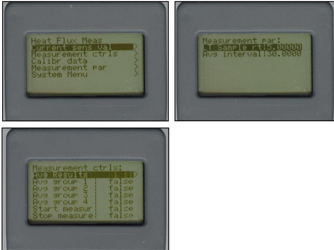
Figure 8.2.2.1 activating the measurement via the Keyboard Display
