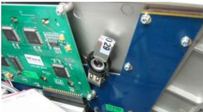
Figure 16 – Installation of USB Memory Stick
