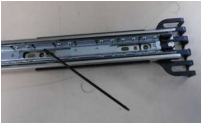
Figure 100 – Attach Rack Mount Adaptors to Outer Slides
