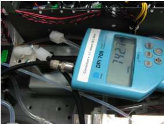
Figure 79 – Disconnect inlet of Photometer
