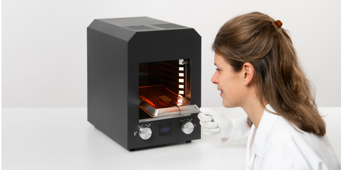
Figure 0.2 Model FHF06 high temperature foil heat flux sensor being used to monitor the performance of an oven. The sensor can be continuously used for temperatures up to T = 250\text{ }^{\circ}\text{C} .
