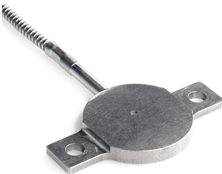
Figure 0.1 IHF01 industrial heat flux sensor
