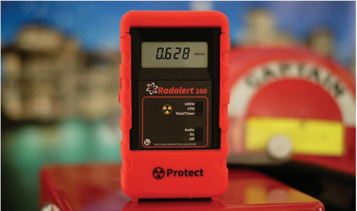
First Responders appreciate the Radalert 200 slide switches - Intuitive and Easy to Operate with firefighting gloves and other PPE.
