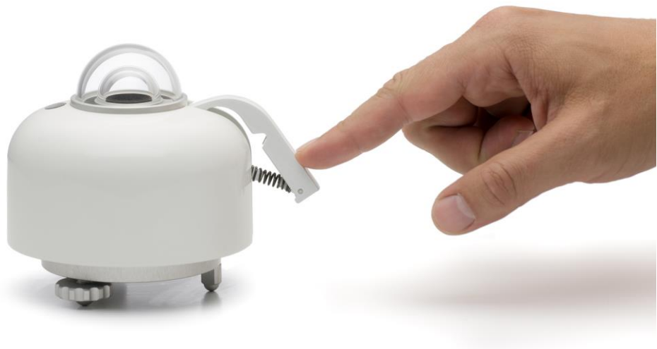
Figure 5.2.2 Installation of SR15-A1's sun screen
