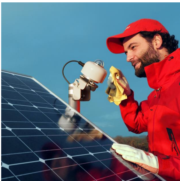
Figure 2 SR15 pyranometer mounted in PoA (Plane Of Array) on a mast for PV performance monitoring
