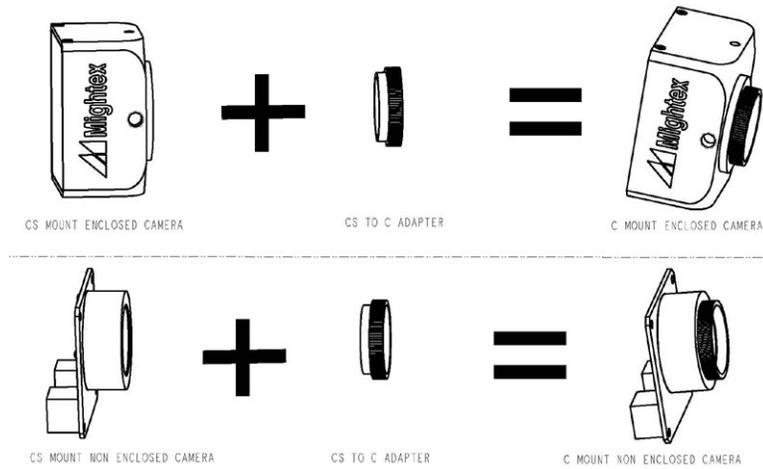
A C-mount camera is composed of a CS-mount camera and a CS-to-C-mount adapter. The latter is essentially a 5mm thick threaded ring.
