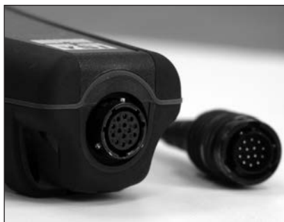
Figure 4, Note the keyed connector.
