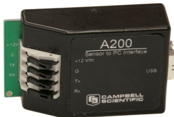
FIGURE 8-1. A200 Sensor-to-Computer Interface
