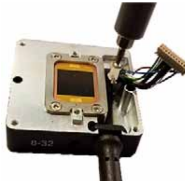
Figure 3-10. Unscrew the Ground Lug
