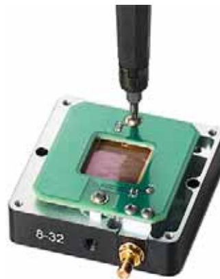
Figure 3-16. Attach Pass-Thru Circuit Board
