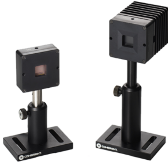
Figure 2-14. Sensor on Post-and-Stand Assembly
