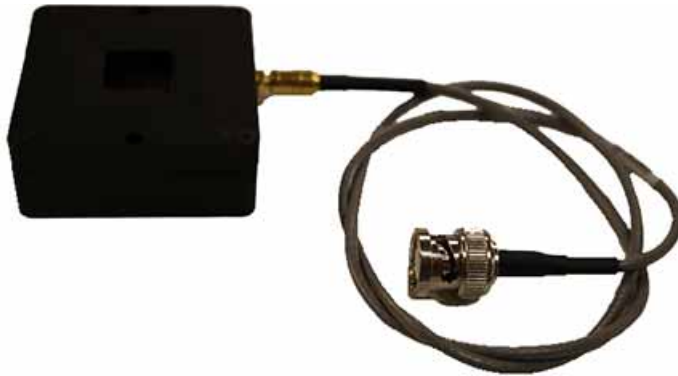
Figure 3-18. Attach SMB Cable
