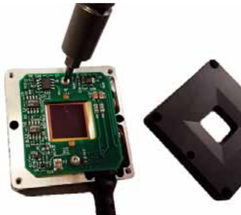
Figure 3-7. Unscrew the Circuit Board
