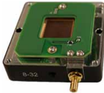
Figure 3-15. Align Pass-Thru Board in Sensor Housing
