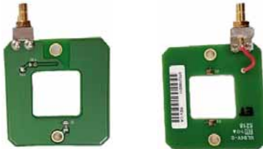
Figure 1-26. Pass-Thru Circuit Board (Front and Back)
