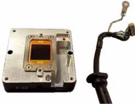
Figure 3-11. Remove Wiring Assembly from the Sensor
