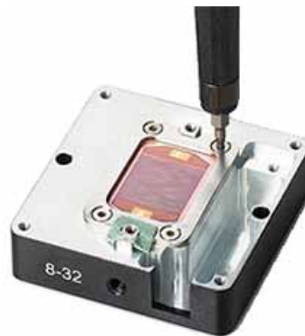
Figure 3-21. Remove Sensor Retainer (Frame)
